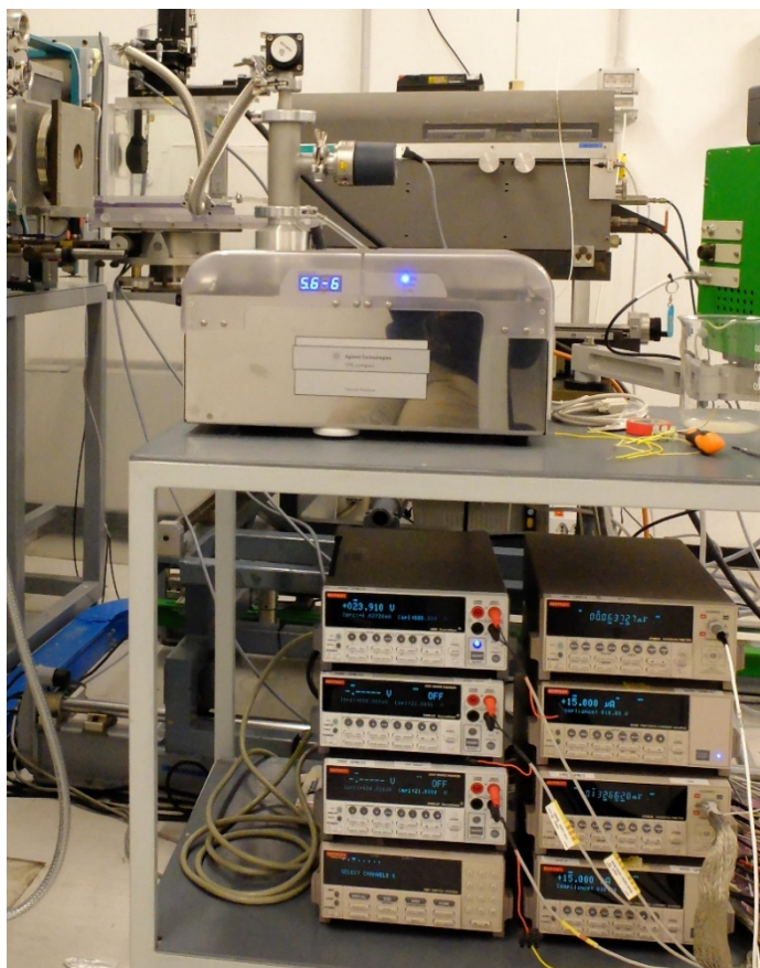
Fig. 1.3: Representation of the technique and instruments used for the ENEA graphite calorimeter primary standard for kV x-rays. Measurements for the present project were done at 2 cm in water and SSD equal to 98 cm (The photograph shows the experimental setup at ENEA at an SSD of 70 cm).
